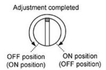
When there is distance fluctuation between proximity sensor and the target, please adjust 2 at the farthest distance from this unit.
