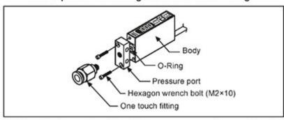
It is able to use it without the pressure port according to environment. In this case O-Ring between pressure port and its body should not be taken out in order to prevent pressure leak.
