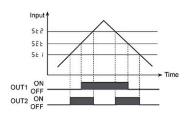
Note1) If it is not enough for difference of sensing level between 5£ 1 and 5£2, £r3 will be displayed. Please set again after applying enough pressure.
