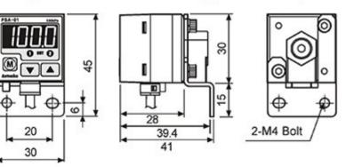
Fixing bracket B for mounting(PSA Series)
