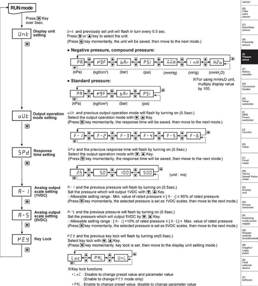
When advance to parameter setting mode and preset setting mode, it displays "Setting item" and "Previous setting value" by 0.5 sec. turn. This display will stop by pressing v or key(Display setting value), if any key is untouched for over 1 sec., it will display old value by 0.5sec. turn again.
