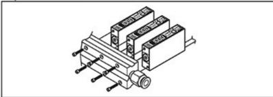
Please connect it by using spanner(10mm) at pressure port in order not to overload on the body when connecting one touch fitting.
