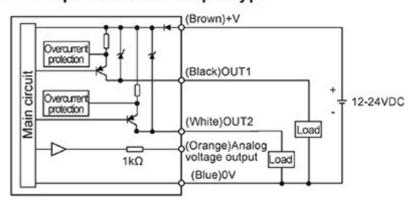
\*\*There is no short-circuit protection in analog voltage output. Do not connect this output to power supply or capacitive load directly.
